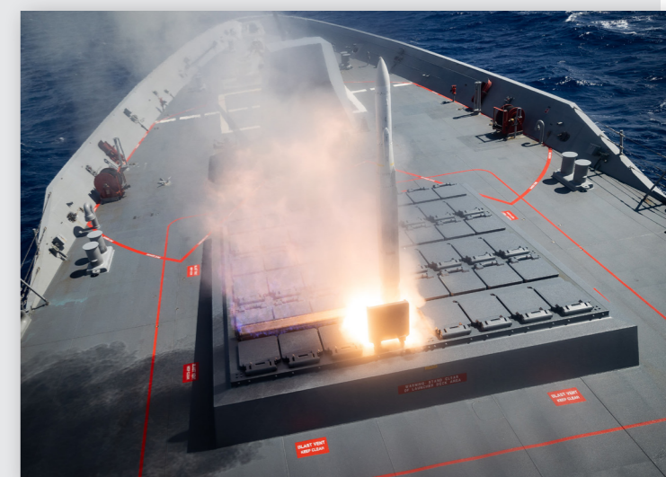
ABOVE: ESSM firing from the Mk 41 VLS on the destroyer HMAS Sydney. Image: ADF
