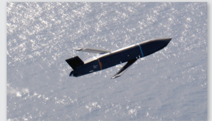
RIGHT: An LRASM skims across the ocean during a test flight. Image: US Navy
