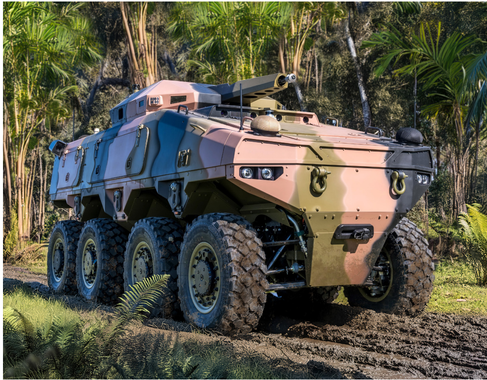
ABOVE: The ATLAS CCV is equipped with a 25mm gun turret, 8x8 mobility and an advanced autonomy and command, control and communications suite.
