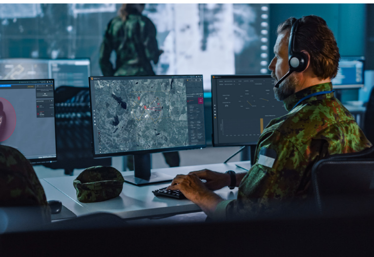
LEFT: A command and control platform that integrates both own and third-party C-UAS sensors and effectors to provide C-UAS awareness and reporting, DroneShield-C2 allows for remote access to deployed DroneShield systems to check status, configure settings, monitor threat levels and respond in real-time. Image: DroneShield
