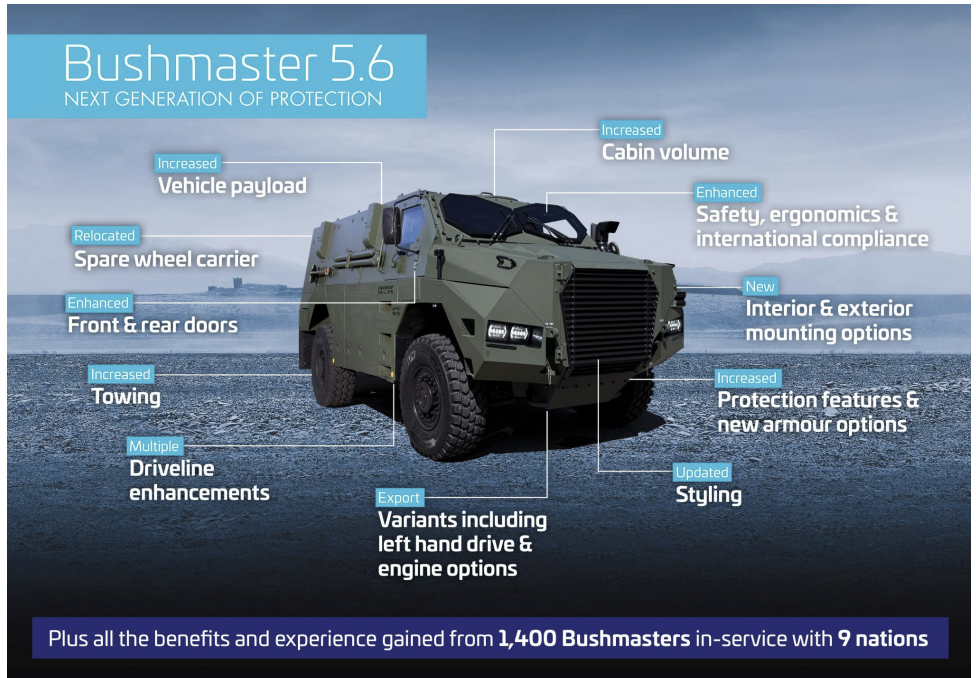
ABOVE: From 2027, the Australian Army will begin receiving the next-generation Bushmaster 5.6 variant, with deliveries at a rate of approximately 40 per year.
