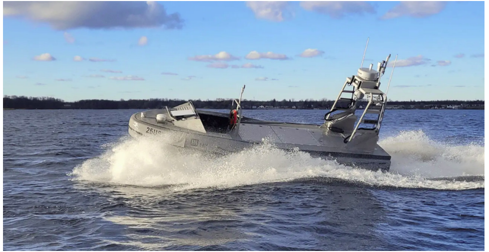
ABOVE: HII delivered two Romulus-25 USVs to the USMC last December, whereupon they underwent at-sea testing and conducted autonomy demonstrations. Image: HII
