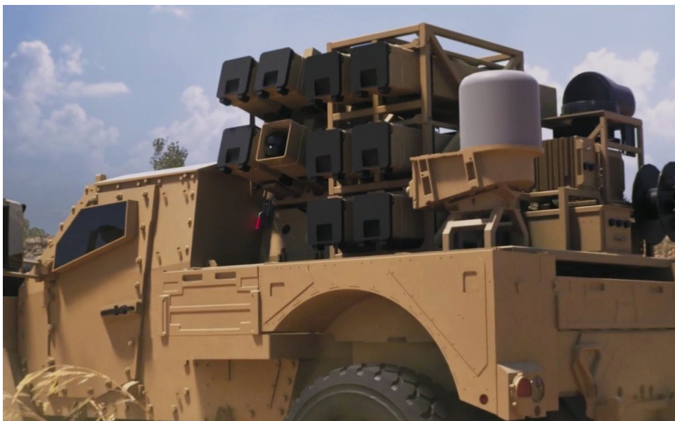
ABOVE: The palletised launcher module contains four ready-to-fire rounds of L-Spike 4X plus six reloads. Previous integration studies by Rafael have confirmed that the module would fit on the rear tray of the Hawkei two-door variant. Image: Rafael
