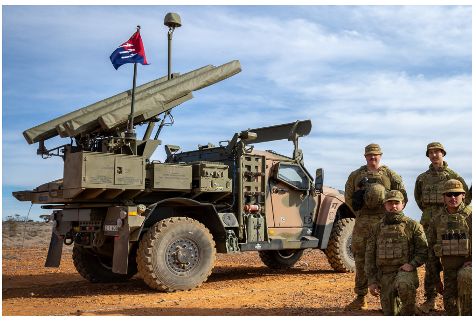
BELOW: The Army is already using Hawkei as a weapons carrier, having integrated the NASAMS High Mobility Launcher onto the rear tray of the two-door variant under Land 19 Phase 7B. Image: Aust DoD
