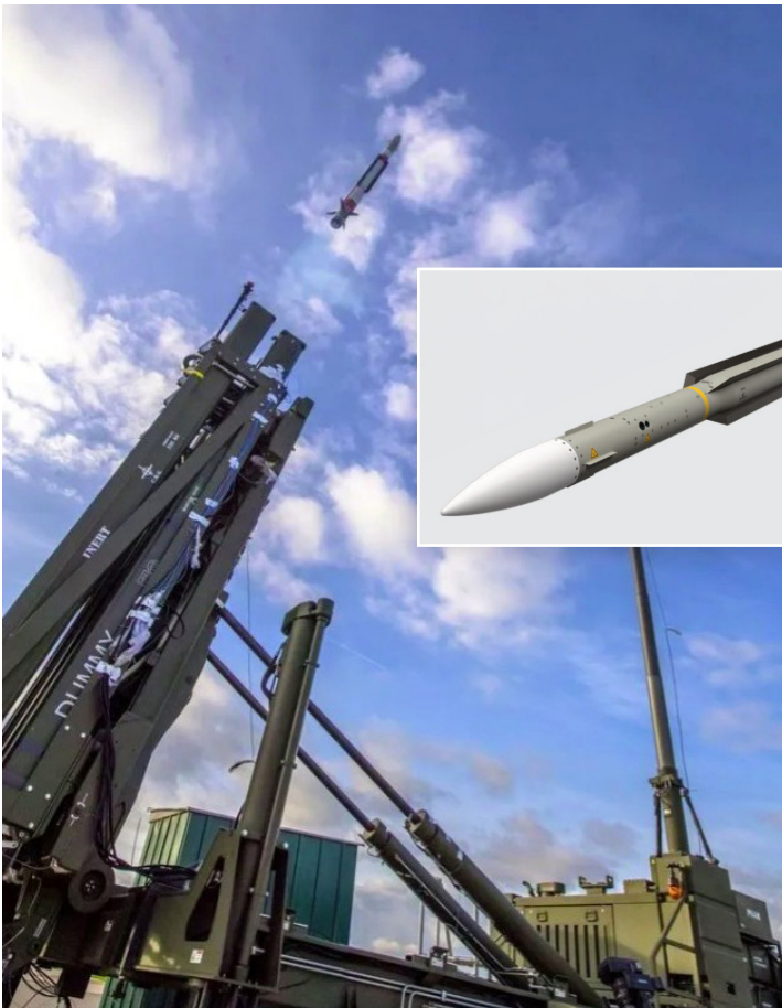
ABOVE: CAMM-ER (and inset) is entering service with the Italian Army as a truck-mounted SR/MRGBAD system known as Grifo. Images: MBDA
